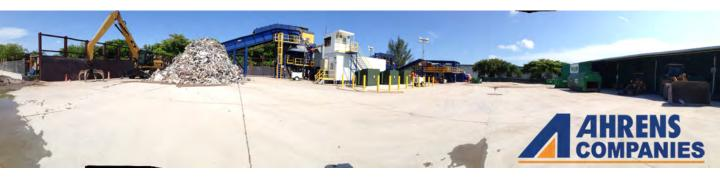
The Sun Recycling Center facility had been dealing with cracking and failing slabs due to the heavy traffic from their metal scrap business. Sun Recycling contacted Ahrens Companies seeking a more resilient concrete slab design. Aware of the benefits of Helix Micro-Rebar, Ahrens turned to Helix Steel for the solution. The Helix engineering team reviewed the initial design of a 6 1/2" thick concrete slab, reinforced
