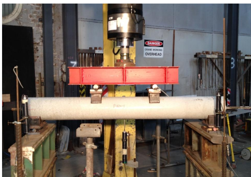
Fig 2. Test setup for a pile specimen with L_0 = 1.5\text{m} and a = 0.5\text{m}
