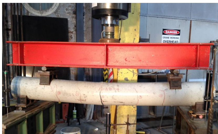
Fig 9. Pile specimen P-N16-4 at failure ( L_0 = 1.5\text{m} , a = 0.2\text{m} )
