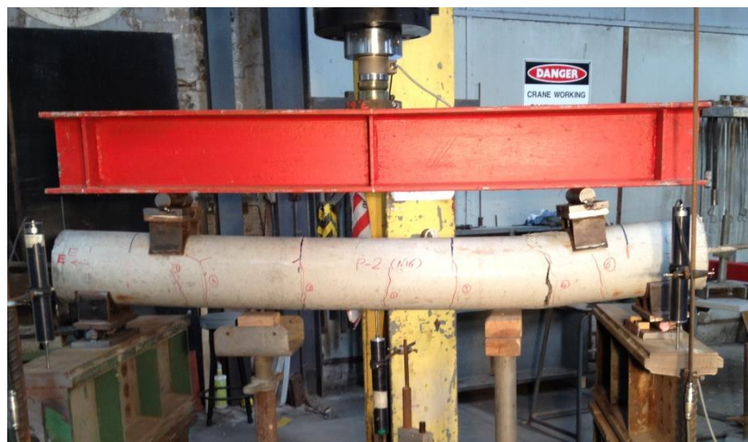
Fig 8. Pile specimen P-N16-2 at failure ( L_0 = 1.5\text{m} , a = 0.2\text{m} )
