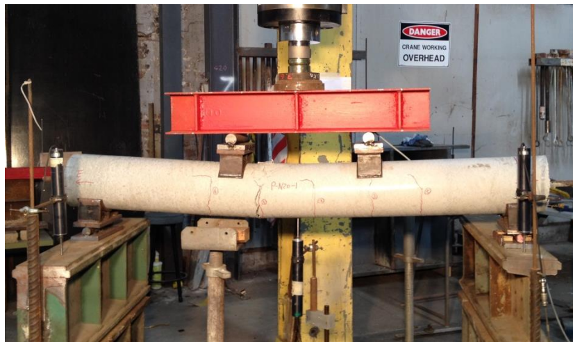
Fig 10. Pile specimen P-N20-1 at failure ( L_0 = 1.5\text{m} , a = 0.5\text{m} )
