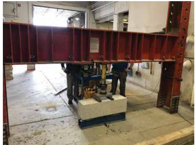
Fig. 1: ASTM C78/C78M flexural test setup
